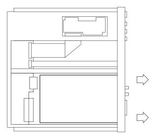
Figure 6–3: Withdrawing the module (Decoder board)
