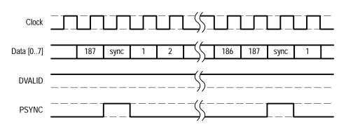
Transmission format with packets of 188 bytes
