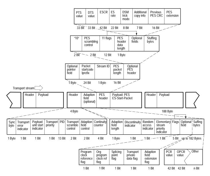
Figure 2–1: Elements of the transport stream syntax
