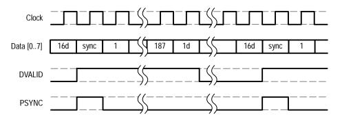
Transmission format with packets of 188 bytes and 16 dummy bytes (= 204 bytes)
