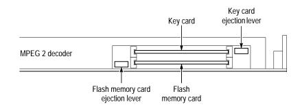
Figure 3–1: Slot for key card
