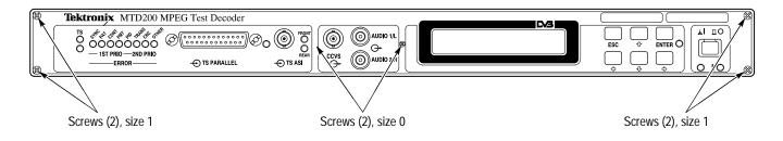
Figure 6–2: Front–panel screws
